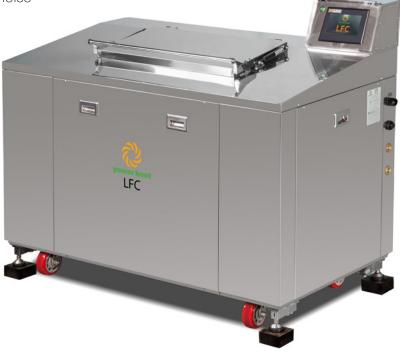
The LFC-200 is a fully enclosed automatic biodigester that safely disposes of 200–360 kg (440–800 lbs) of waste food each 24 hours with no noise or odor. Once installed, you can add waste at any time without needing to empty byproducts. The LFC discharges only decomposed food as grey water that is environmentally safe.
