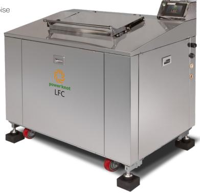
The LFC-100 is a fully enclosed automatic biodigester that safely disposes of 100–180 kg (220–400 lbs) of waste food each 24 hours with no noise or odor. Once installed, you can add waste at any time without needing to empty byproducts. The LFC discharges only decomposed food as grey water that is environmentally safe.
